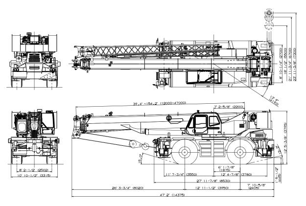
Note : Dimension is with boom angle at -1.5 degree.
