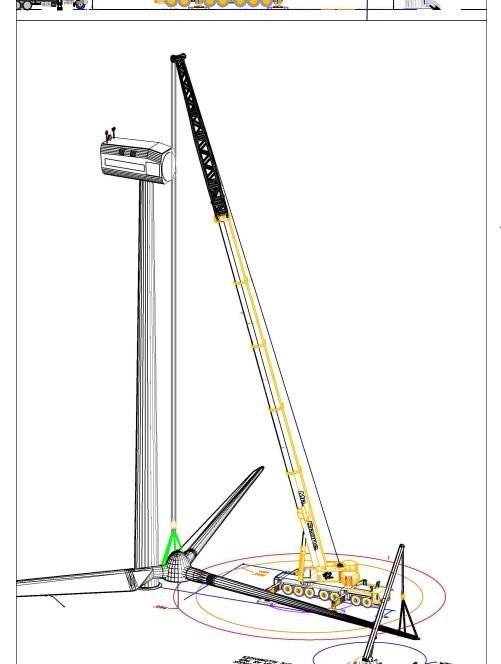
LTM1400-7.1 TRUCK CRANE 169' MAIN BOOM 69' FIXED JIB 132,000 LBS CTWT **FULL OUTRIGGERS**
