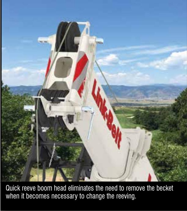
Quick reeve boom head eliminates the need to remove the bucket when it becomes necessary to change the reeving.
